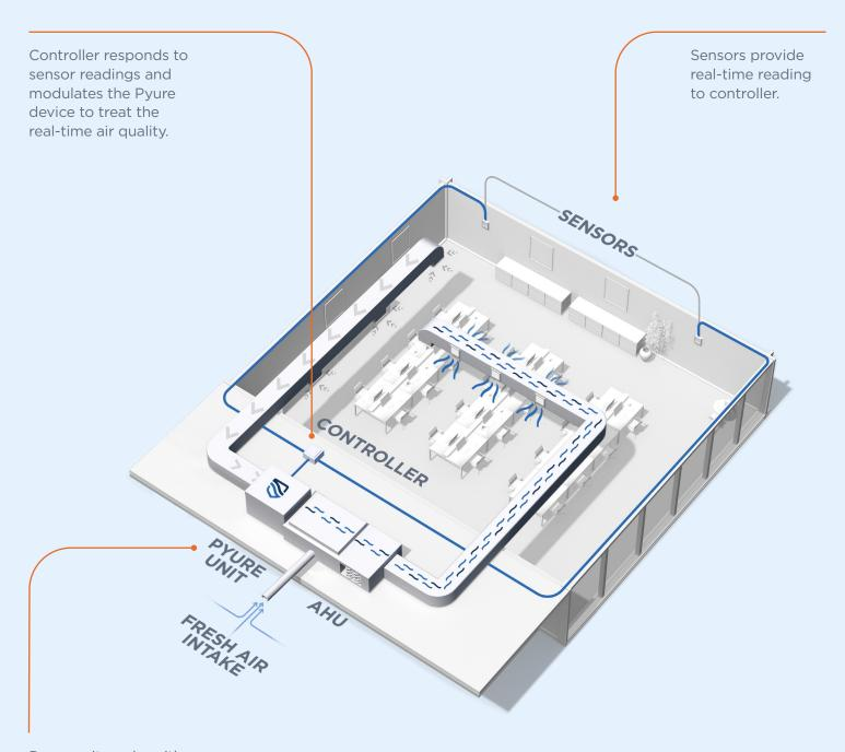
Pyure unit works with single or multiple air handling systems.
